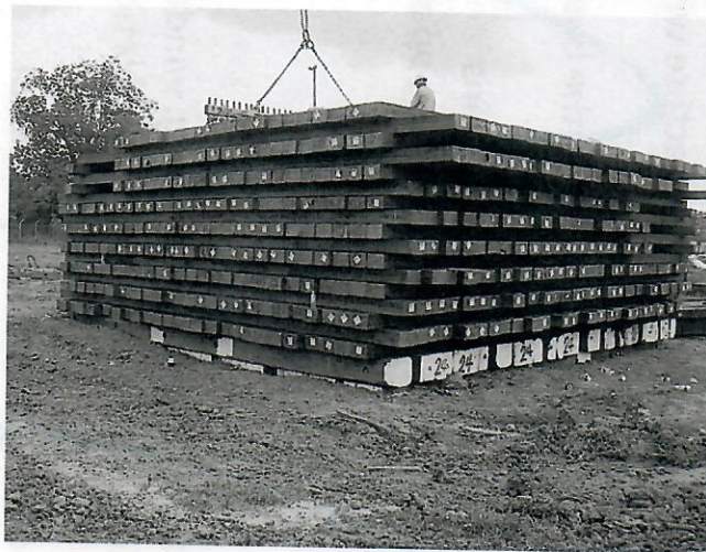
Cell A fully loaded with 1100 tons of steel
