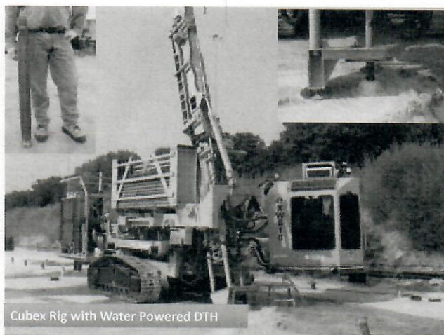
Figure 1. Water Powered Down-the-Hole Hammer mounted on a Cubex rig. (Courtesy of ACT Ltd.)
