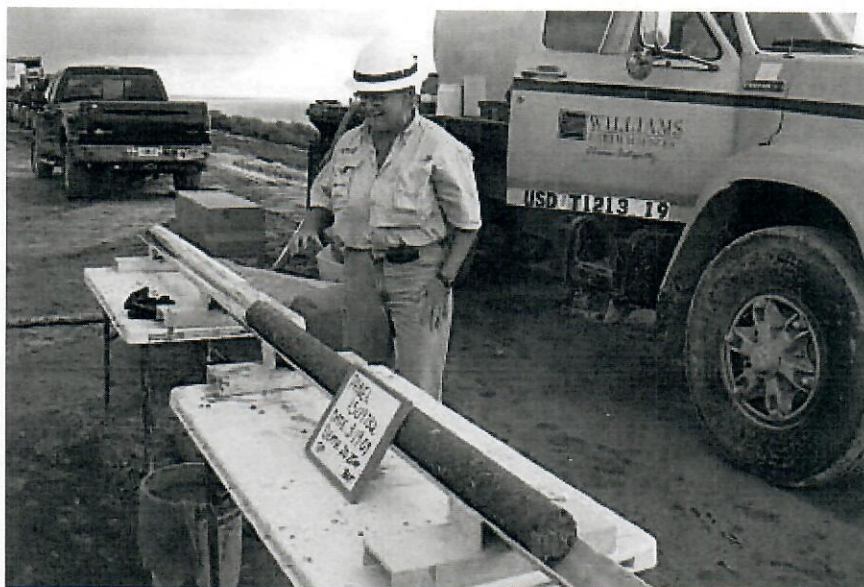
Photo 7: Typical core extracted from DM cutoff at Herbert Hoover Dike, FL.
