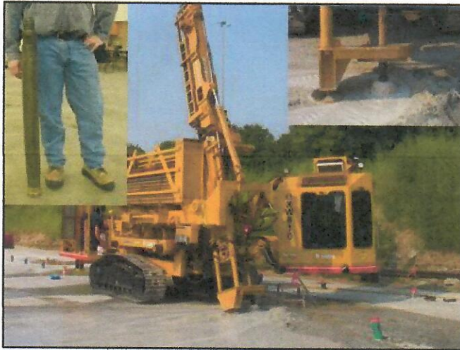
Figure 3. Photo of rotary percussion drill with water activated Down-the-Hole Hammer (Upper Left).
