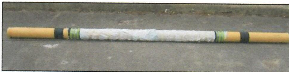
Figure 5. MPSP standpipe with barrier bag.
