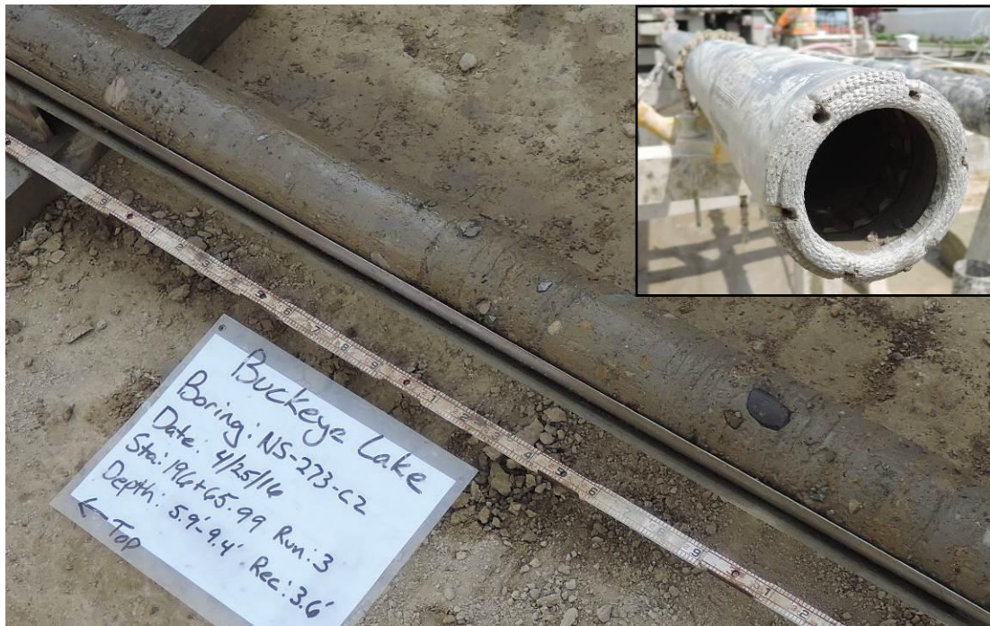
Figure 6. Good core recovery of soil-cement mixture with coarse sand and gravel in a weak matrix, with inset showing side discharge core bit.
