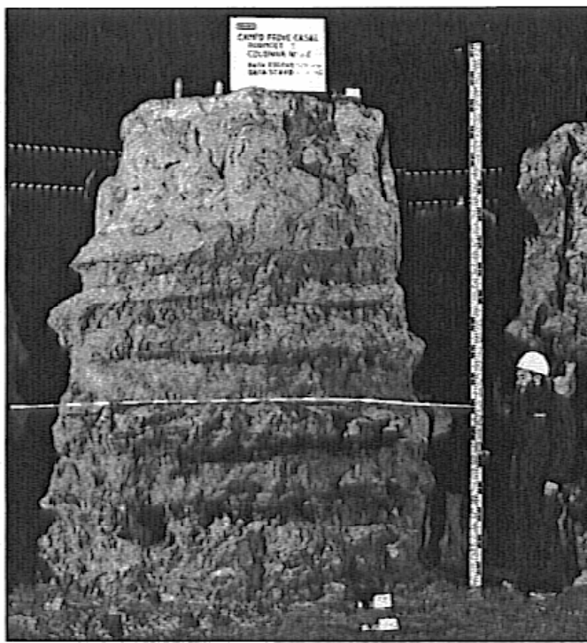
FIGURE 32. Rodinjet 3 column in variable alluvial materials excavated 9 days after grouting.
